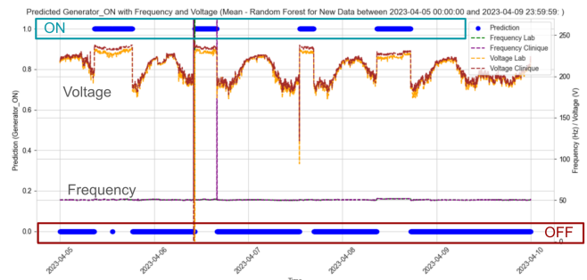
Figure 5. Voltage, frequency, and predicted generator usage at CH Bethesda Ndosho between 5-9 April 2023
